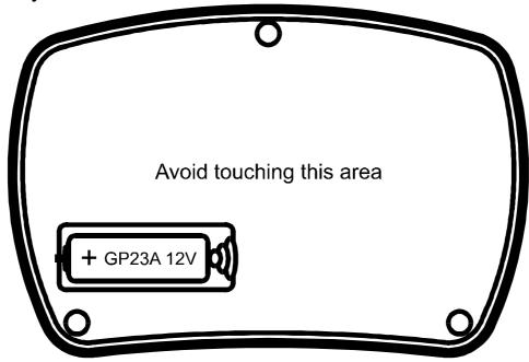
The battery should be replaced with a high quality battery identical to, or equivalent to an Alkaline 23A, V23A, GP23A, MN21 12V (10mm diameter x 28mm length). Carefully replace the rear panel, do not over-tighten the screws.
