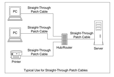
These are generally used for connecting computers hubs (routers or switches) or simply between a PC and wall socket (which eventually connects to a hub).
