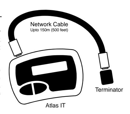
The Atlas IT is supplied with two short patch cables to allow for the testing of network cabling that is accessible only by sockets (or a patch panel). This is illustrated here:
