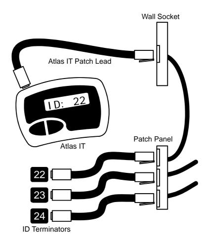
These special terminators can be used in exactly the same way as the standard (non-identified) terminators. They are automatically recognised by the Atlas
