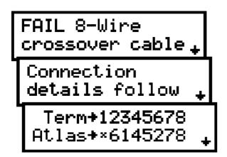
In this example, the closest cable type match is an 8-wire crossover cable. Pressing the **scroll-off** button to view the next pages reveals the nature of the fault.
